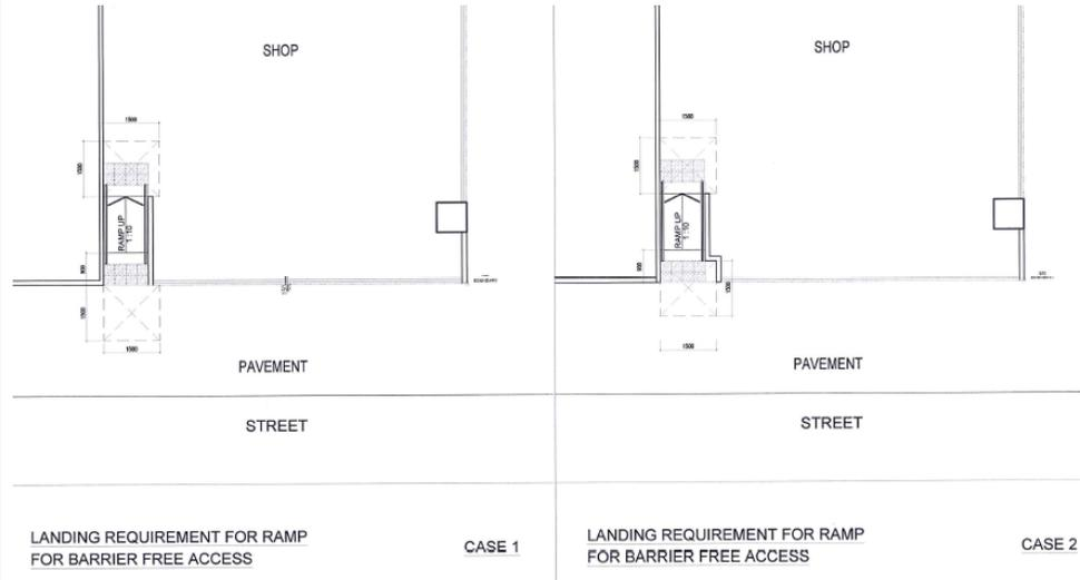
*required provided that such clearance space would be available in the pavement for direct entry to and exit from the building. Notwithstanding this, a clear space within the development of not less than 900mm in depth, i.e. 600mm for tactile warning strip and 300mm for horizontal extension of the handrails as shown in Figures 7 and 16A of the DMBFA 2008 respectively, was still required to be provided at the foot of the ramp.]*
